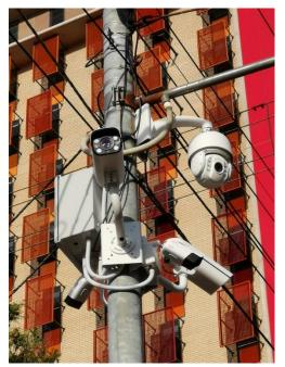
The balled-looking camera that installed to the upper right of the telegraph pole is loaded with features including ultra-low illumination, motion detection, up to 180m IR distance scale and multi-streams. This starlight HD speed dome camera is an excellent choice for ultra-long distance monitoring as it can provide clear views of far distance.
